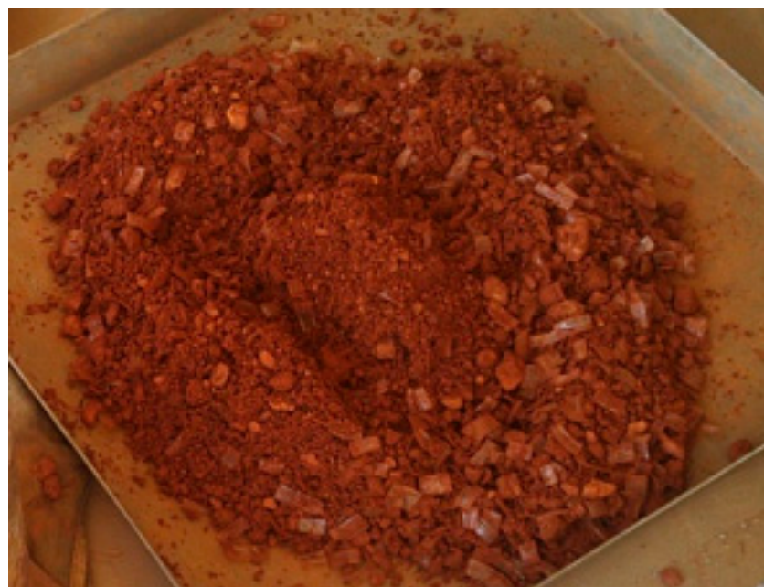
Figure 2. Lateritized plastic (mixture of lateritic soil and shredded plastic waste).
