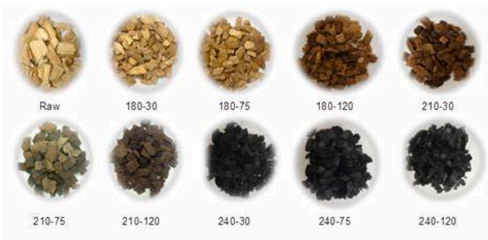
Fig. 13. Colour transformation during Patula pine wood chips' torrefaction [191]. Reprinted with approval from Elsevier (License no.: 5502990269268).
