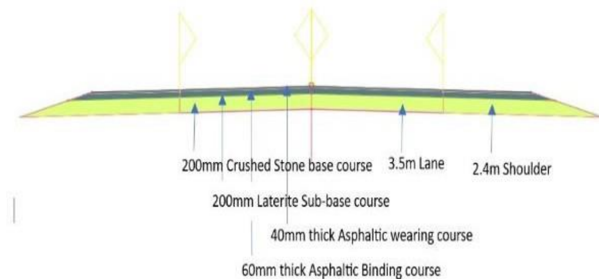
Figure 3. Existing Two-Lane, Two-Way Road Structure of The Western Bypass Road, Abuja, Nigeria.
