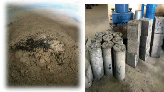
Plate 2: Mixing and casting of steel fiber reinforced concrete samples
