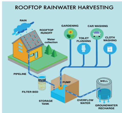
Figure 6: Layout for rainwater harvesting(50)
