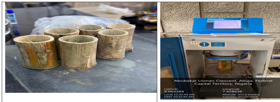
Fig. 2. Compressive strength test specimens and set up.
