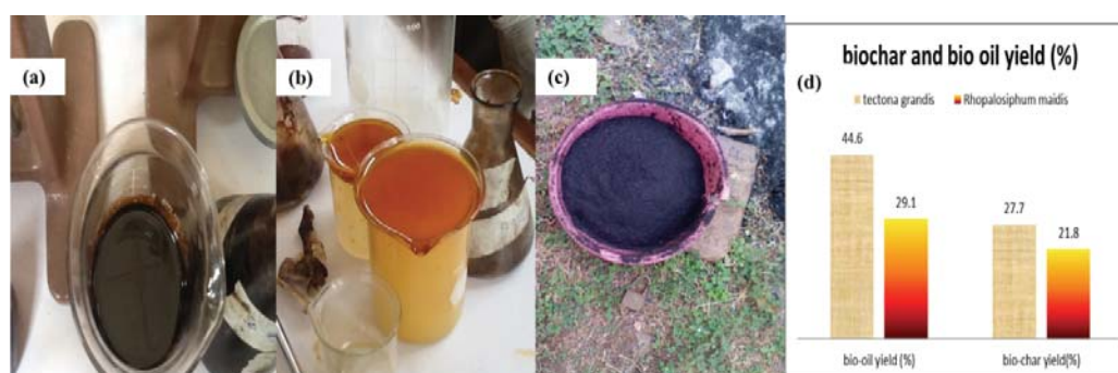
Fig 3: (a) bio-oil crude. (b) bio-oil distillates. (c) bio-char yield. (d) % yield of bio-oil and bio char.
