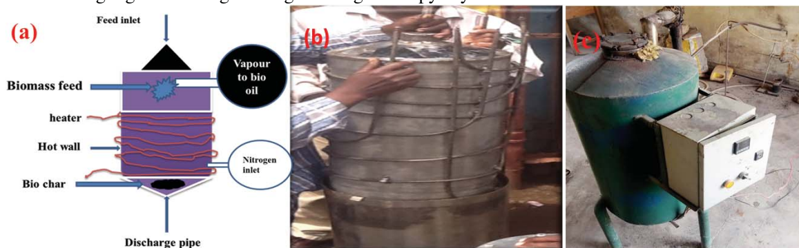
Fig 1: (a). Schematic of heat transfer method in ablative pyrolyser (b). Heater wound round the stainless steel (c). Full assembly system of the pyrolysis reactor
