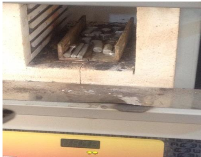
Figure 2. Samples in furnace during heat treatment.
