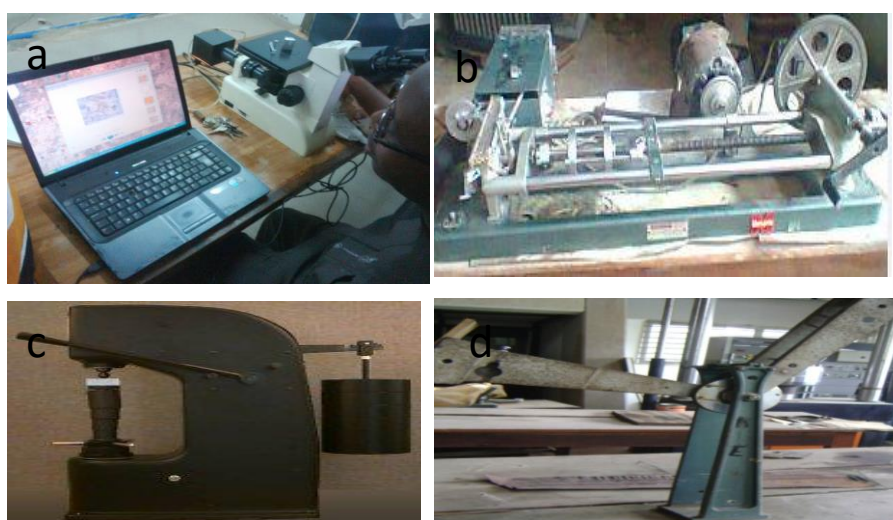
Figure 3. Experimental set up for (a) Microstructural test (b) Tensile test (c) Hardness test (d) Izod test for impact energy.
