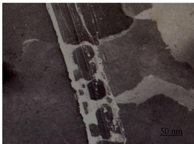
Fig. 3. Scanning electron micrograph of bare aluminium specimen exposed to 100% relative humidity at 313 K for 480 h.
