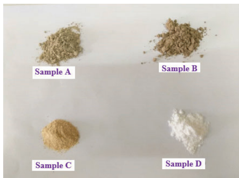
Figure 1: Raw Trona (Sample A), Calcined Trona (Sample B), Extracted Soda ash (Sample C), Imported Soda ash (Sample D)
