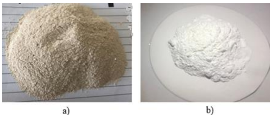
Figure. 1. Eggshell before and after calcination: a) UCES; b) CES
