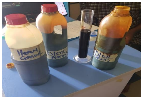
Figure 1: Refinery intermediate products (Decant oil, Heavy gas oil, light cycle oil)
