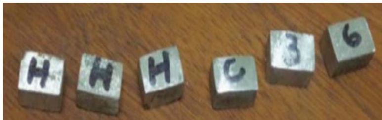
Figure 4: Micro hardness test specimen
