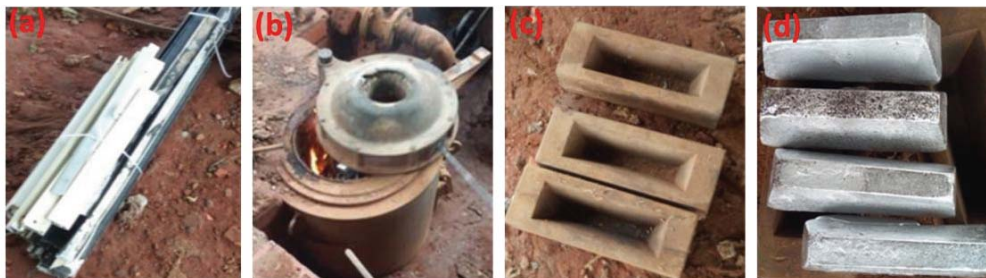
Figure 2: (a) Scrap of Al 6063 alloy (b) Crucible Furnace (c) Ingot metallic moulds (d) Billets of Al 6063 alloys
