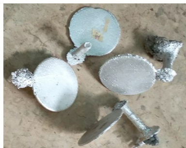
Fig. 1. Solidified wear sample.
