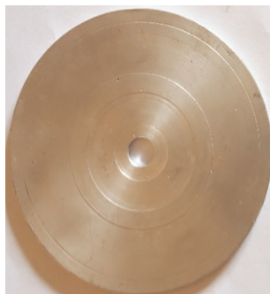
Fig. 2. Typical example of machined wear sample.
