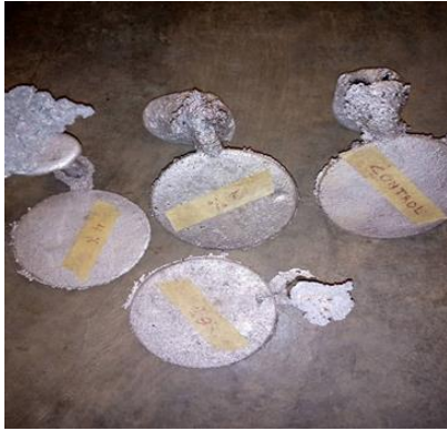
Fig. 2 AMCs produced at various weight percentages (0, 2, 4, and 6 wt.%) of OCA
